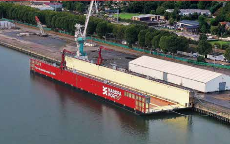
NB04 ABU DHABI FLOATING DOCK 10.000 TLC - 180 x 30 m
