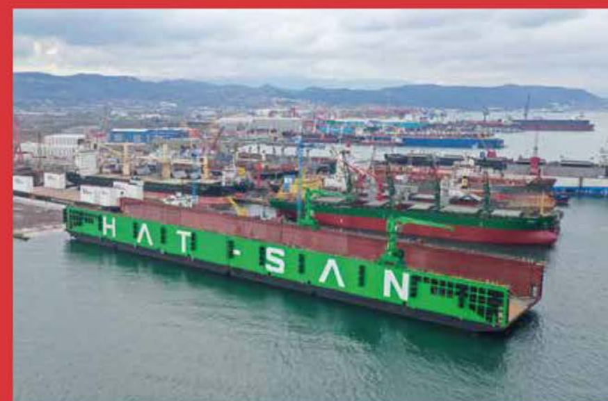
NB18 HAT-SAN FLOATING DOCK 25.000 TLC - 250,5 x 38 m
